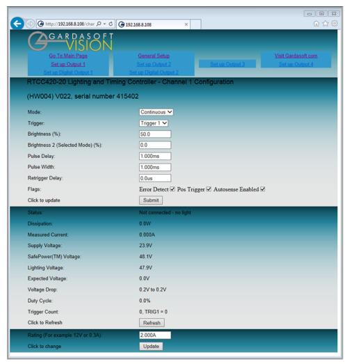
You can set up all the parameters for each output channel. Pressing the **Submit** button updates the RTCC configuration and saves the changes to non-volatile memory. On this page you can:
